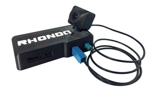
Rhonda H22 System On Module – based GMSL2 evaluation kit provides an end-to-end setup for video capture by up to 2 camera modules, GMSL2 transmission via up to 15m cables with almost zero latency, processing on SOC and output to host device. H22 SOM is a low-power, ready-to-integrate and ready-to-production hardware platform for robotics and micromobility applications.
